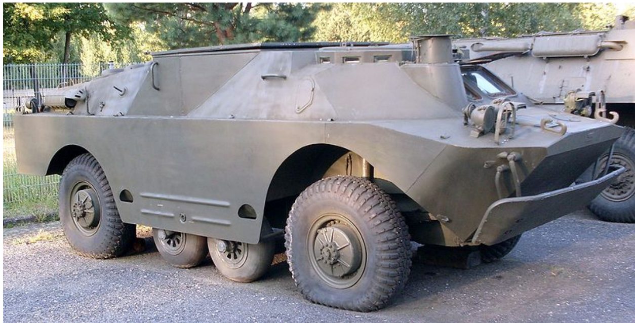
Figure 4. Belly wheels deployed on a BRDM-1U
