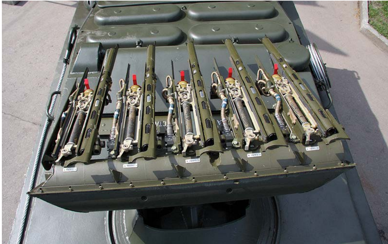
Figure 16. 9P148 Konkurs reveals the launcher rails at a static display in Russia
