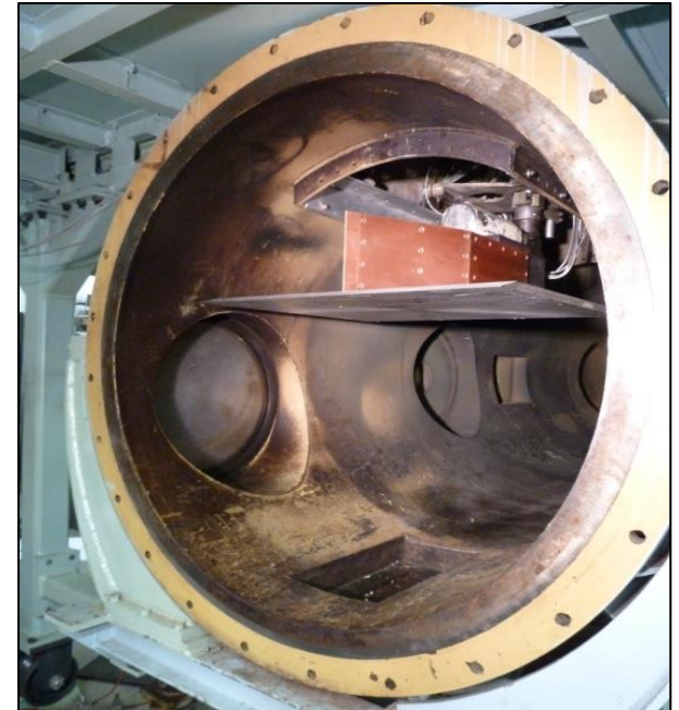
Test article installed in AHSTF with bulkhead and nozzle removed
