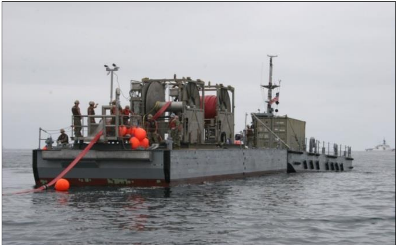
Figure 6.1 Amphibious Bulk Liquid Transfer System (ABLTS)
