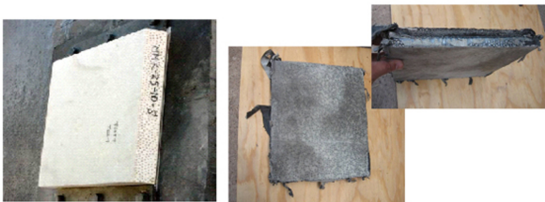
Figure 1. Pre- and Post- Blast
