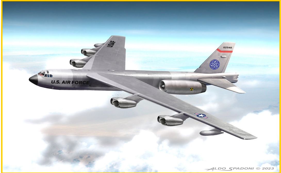
This digital illustration by aerospace artist Aldo Spadoni, of the proposed B-52G Stratofortress with the XNJ140E-1 nuclear powerplant attached to the left side of the bomber, shows how the test configuration may have looked had the nuclear propulsion program continued.
