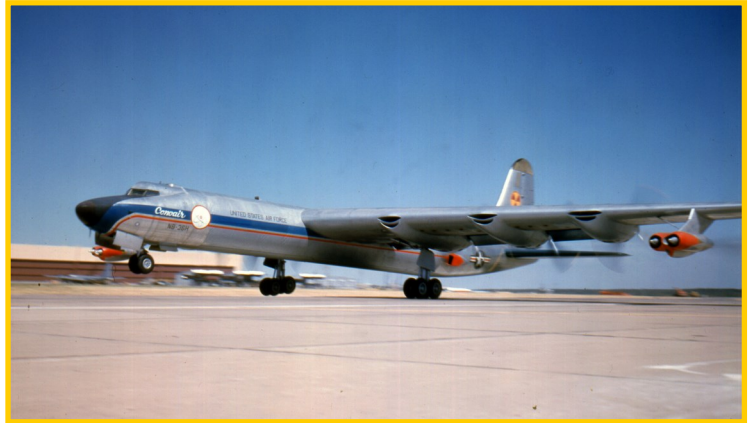
The Convair XB-36H 'Crusader' carried a nuclear reactor aboard the aircraft, though it never powered the bomber in flight. Convair photo.
