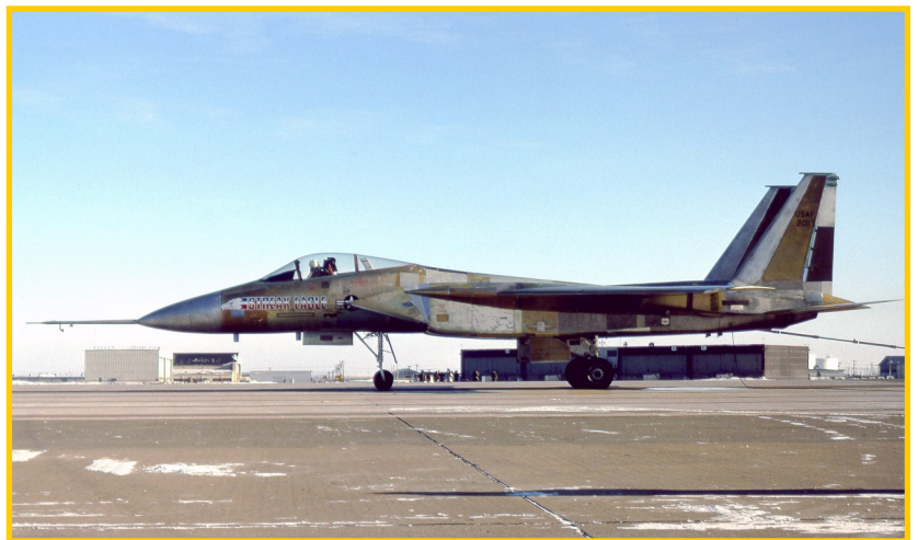
A specialized hold back explosive bolt attached to a steel cable replaced the tailhook for the record attempts. With engines at full power, the pilot released the aircraft and reached rotation speed in approximately 3 seconds.
