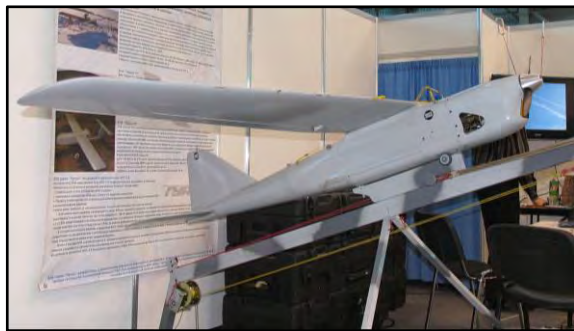
Figure 8. The Orlan series of UAVs is widely proliferated and very capable
