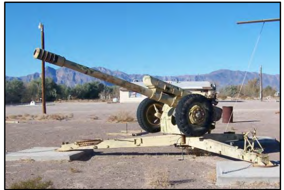
Figure 3. D-30 122mm light towed howitzer
