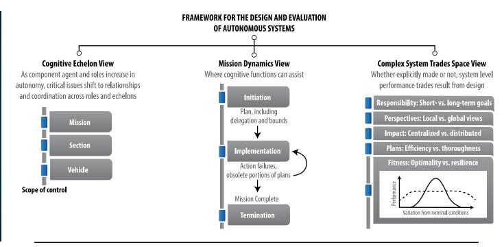
An autonomous system reference framework highlights the allocation of cognitive functions between the human operator and the computer. *The Role of Autonomy in the DoD Systems (2012)*.
