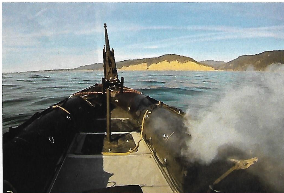
In tests off the California coast, the Lockheed Martin Area Defense Anti-Munitions laser system burns through the hull of a military-grade boat.
