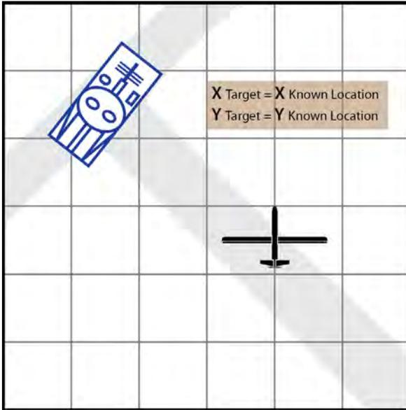
**1st Method-** Use of a reference point. This method can be used if the coordinates of a given reference point (landmark or intersection) are known. The disadvantage of this system is that the coordinates of the reference point must be known with certainty, requiring detailed maps and/or GIS data. In addition, target accuracy diminishes the farther the target is from the reference point. Conclusion: This method works, but is the least suitable for artillery spotting.
