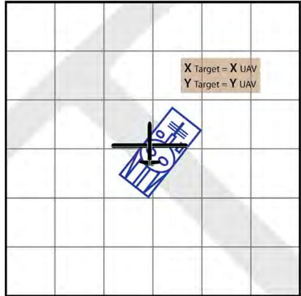
**2nd Method-** Fly above the target. The UAV flies above the target and its position is recorded. Target accuracy depends on the accuracy of the UAV's navigation system. The disadvantage of this method is that it requires flying over the target, meaning that only a limited number of targets may be acquired and that the UAV is extremely susceptible to enemy fire. Conclusion: This method works, but is most suitable for less organized adversaries, such as insurgents.
