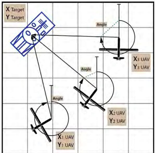
**4th Method-** Use of multiple azimuths. The UAV takes several azimuths on a given target, while in flight. Trigonometry is then used to calculate the position of the target. This method provides good accuracy and the capability to acquire many targets. This method requires a sophisticated UAV, but is completely passive, an advantage that can significantly increase the UAV's life expectancy above the modern battlefield. Conclusion: this is preferred method for UAV artillery spotting.
