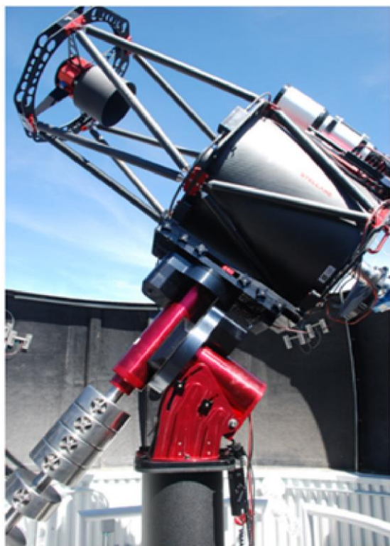
The FALCON Telescope install in Chile with the tubular structure and the German mounting system. (Courtesy of J. Nilo)
