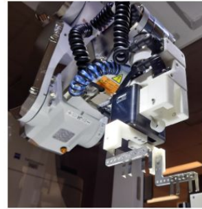
BAB Pick n' Place tool (i.e., the grippers)
