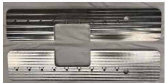
Fig. 5 New side plates for transonic cascade with cutouts for schlieren access
