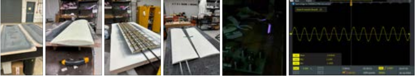
Figure 3 From left to right: molds for making wing skin; wing skin made from composite material; assembling wing skeleton; wing section before gluing the suction surface; test of DBD actuator and test of microphone pressure sensor.
