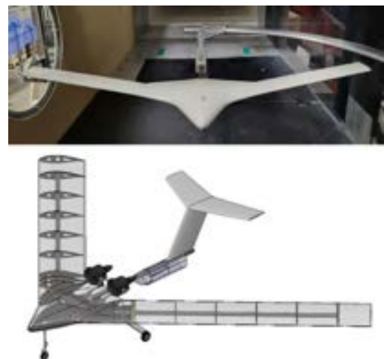
Figure 2: Top) Scale model in ALSWT. Bottom) New design with 45° wing sweep
