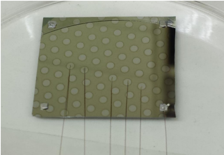
Wire contacts: Silver paint / conducting epoxy / indium dots
