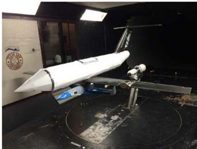
Figure 2. Supersonic aircraft demonstrator attached to mothership
