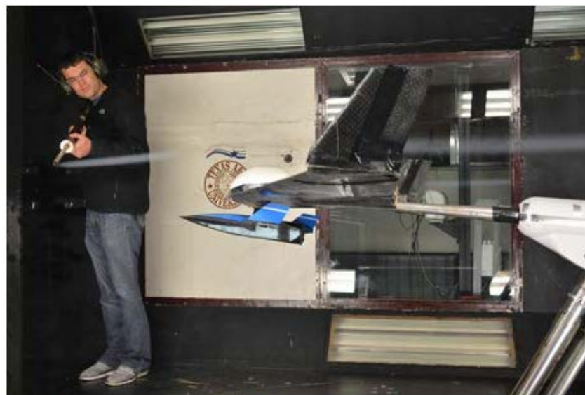
Figure 3. Supersonic aircraft demonstrator attached to mothership undergoing flow visualization via smoke
