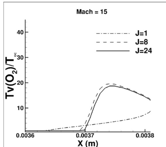
Higher degree of dissociation for higher J resulting in reduced shock-standoff distance
