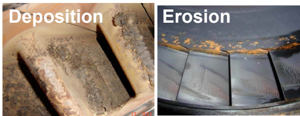
Photos of damaged turbine blades (Bons, 2010)
