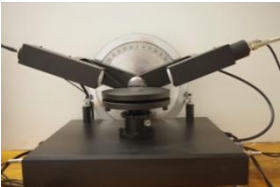
Fig.6. The PHE-102 is a variable angle spectroscopic ellipsometer
