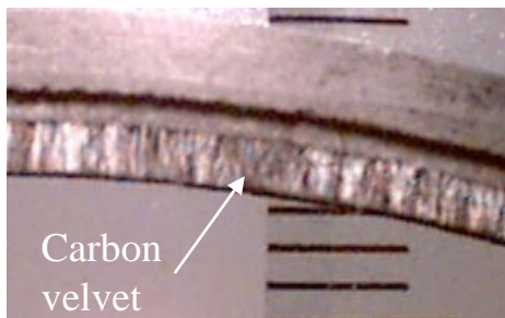
Plasma burned out all protrusive fibers
