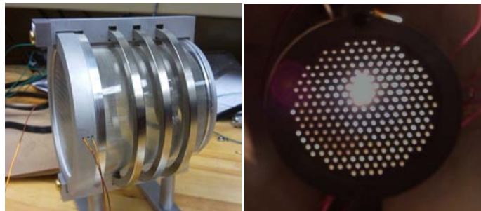
Figure 1. Ion engine simulator with a bare filament cathode and magnetically isolated anode. Ion energies can range from 0 – 500 eV with currents up to ~10 microamps.
