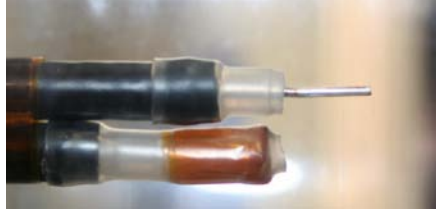
Figure 6: Photograph of dual probes, one probe is shielded from plasma to isolate non-plasma effects.
