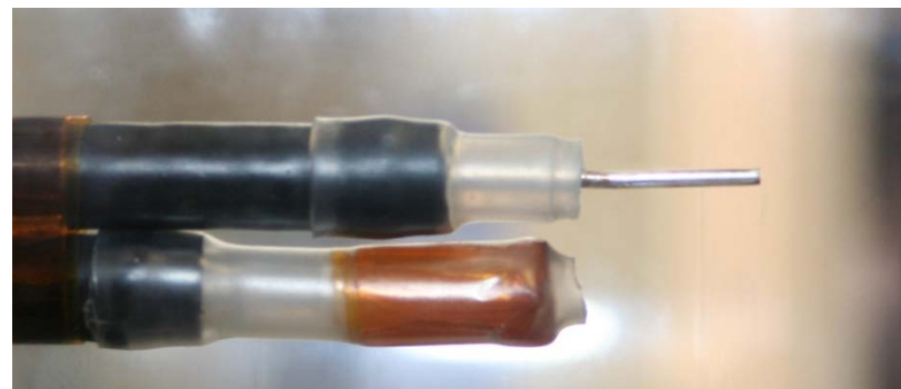
Dual probes used for MPX test article consisting of an exposed probe (top) and a dielectrically shielded null probe (bottom).
