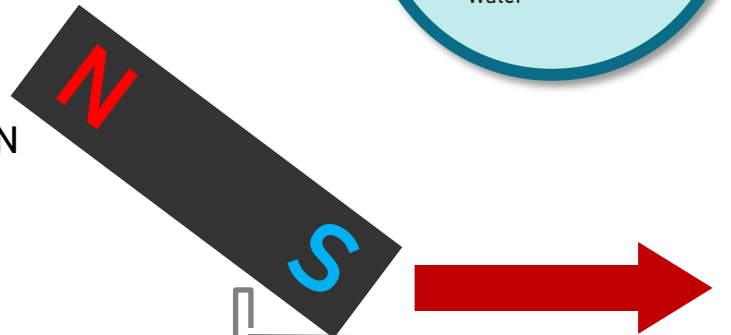
Diagram demonstrating a magnet going along the needle in ONE DIRECTION ONLY .
