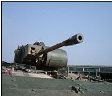
Figure 2. Rheinmetall 30-mm MK 30-2/ABM (air burst munitions) autocannon
