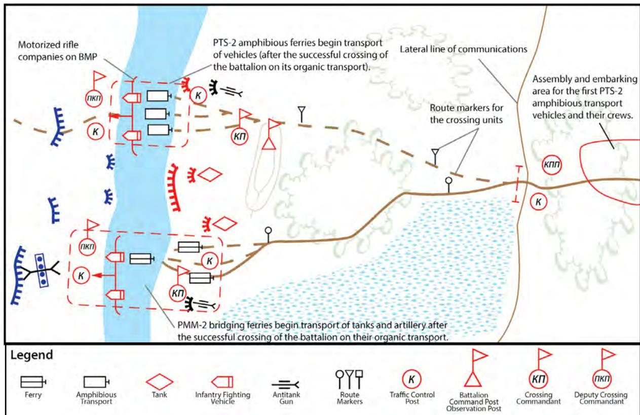
Figure 1. Engineer support of an assault crossing
