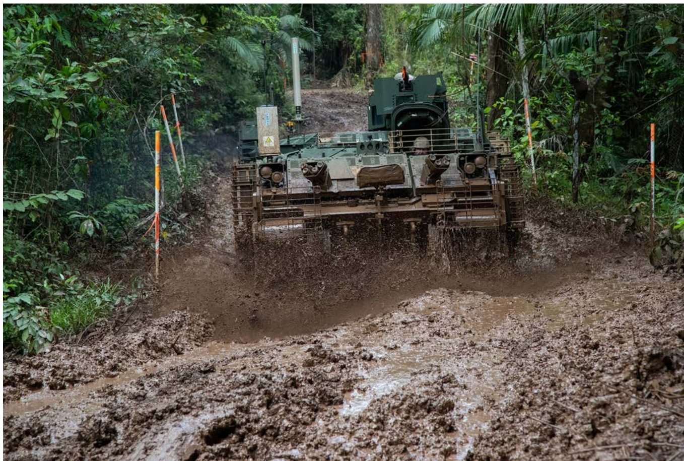
Figure 1. The AMPV has undergone extensive testing at all three of U.S. Army Yuma Proving Ground's natural environment test centers: Yuma Test Center outside Yuma, AZ; Cold Regions Test Center at Fort Greely, AK; and most recently at Tropic Regions Test Center in the jungle of Panama. (U.S. Army photo)
