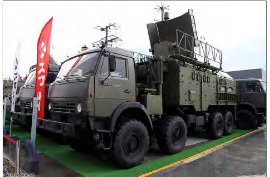
EW The 1L265 Intelligence Vehicle of the 1L267 Moskva-1 System. Source: Vitaly Kuzmin via Vitalykuzmin.net, https://www.vitalykuzmin.net/Military/ARMY-2017-Static-p4/-KG92wV3/A , CC BY-NC-ND 4.0
