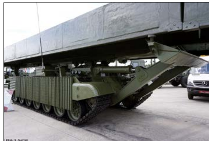
MTU-2020 Armored Mechanical Bridge.
