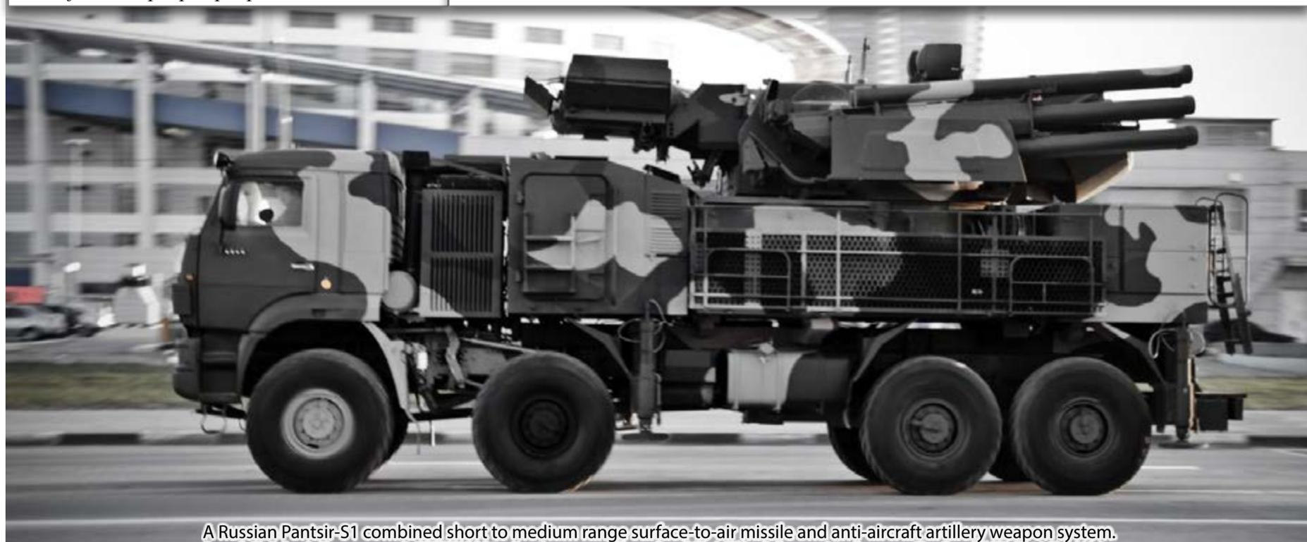
A Russian Pantsir-S1 combined short to medium range surface-to-air missile and anti-aircraft artillery weapon system.
