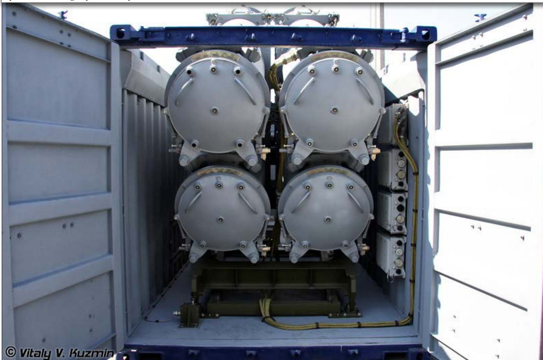
Container missile system Club-K in 20-foot variant with Kh-35UE missile.
