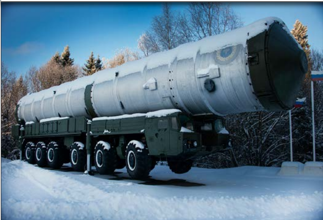
Russian Transport and reloading vehicle on the chassis of the MAZ-547A for long-range intercept missiles 51T6 as part of the Amur A-135 anti-missile defense complex.
