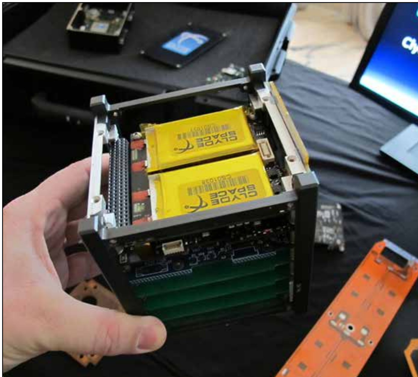
1U CubeSat structure without outer skin; CubeSATS are one of the most popular microsatellite frames because of their standardized configurations.
