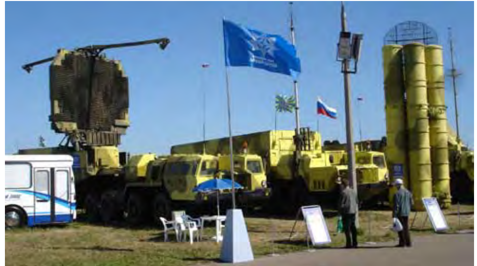
S-300PMU-2 vehicles. From left to right: 64N6E2 detection radar, 54K6E2 command post and 5P85 TEL. by Ajvol [Public Domain], via Wikimedia Commons
