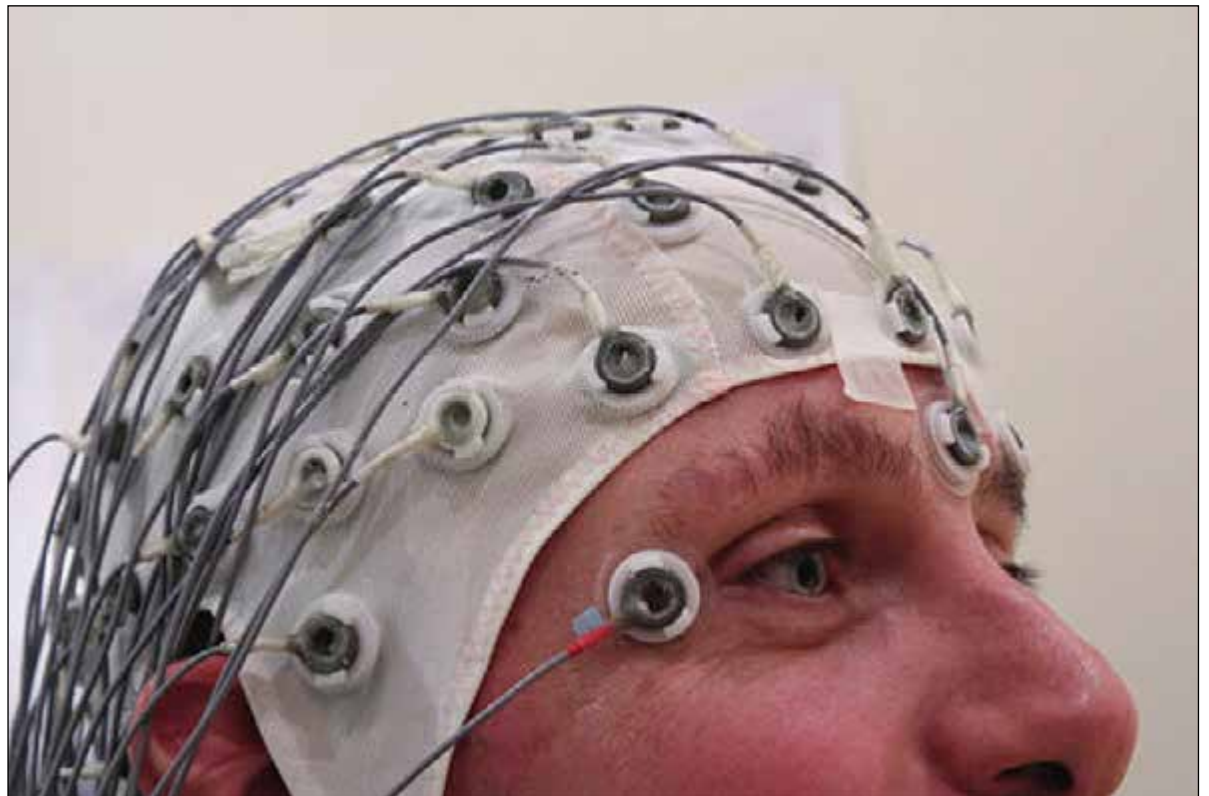
A cap holds electrodes in place while recording an EEG.
