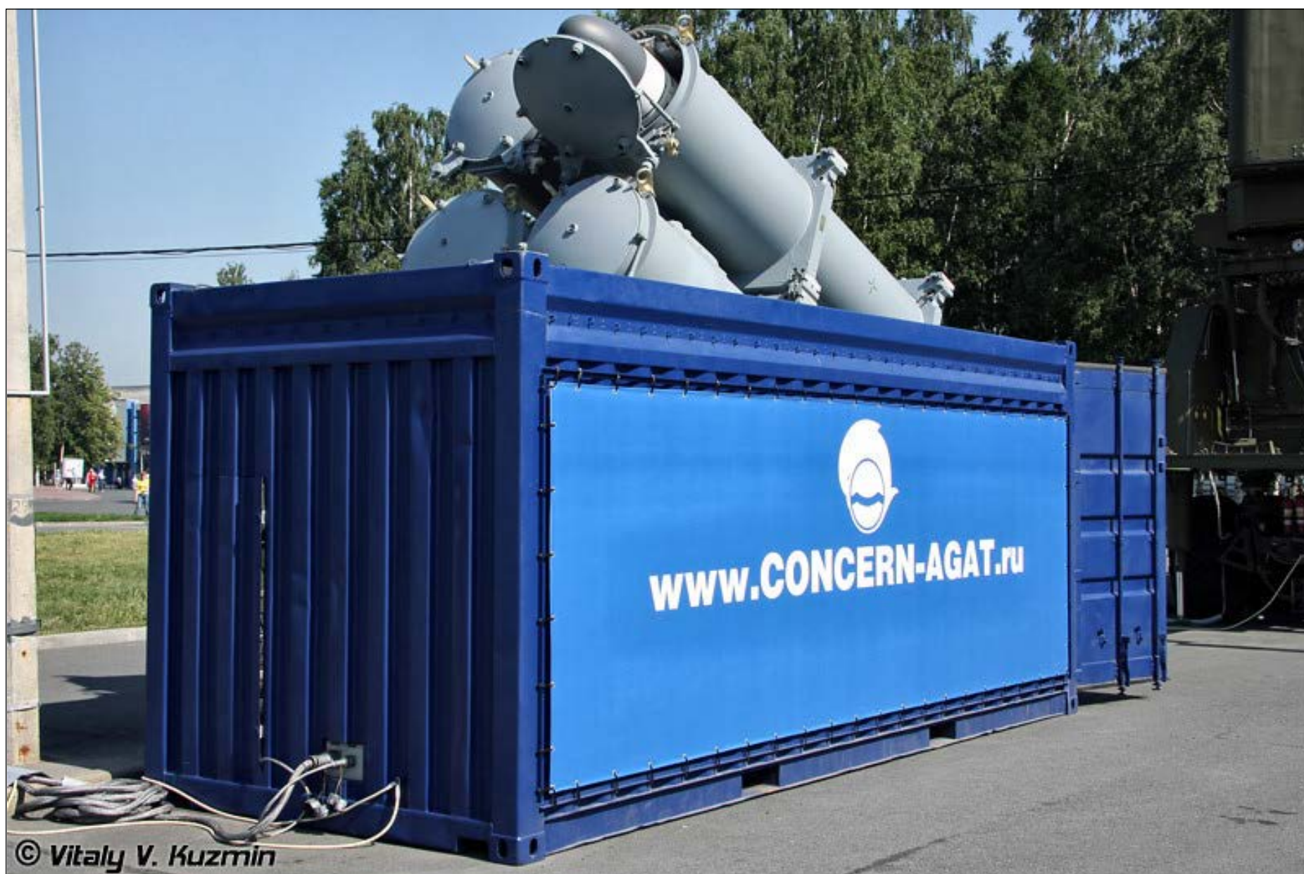
Container missile system Club-K in 20-foot variant with Kh-35UE missile. Source: Vitaly Kuzmin Military Blog, https://www.vitalykuzmin.net/Military/IMDS-2011/i-hwrK7DR , CC 4.0.
