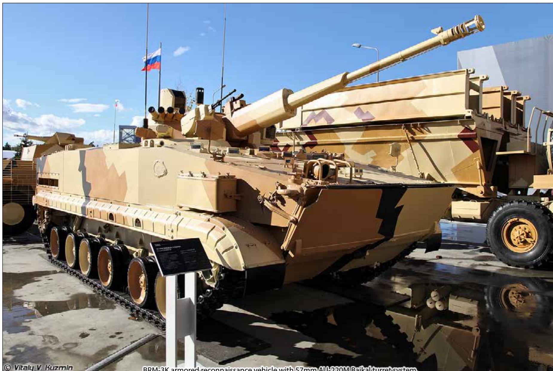
BRM-3K armored reconnaissance vehicle with 57mm AU-220M Baikal turret system.
