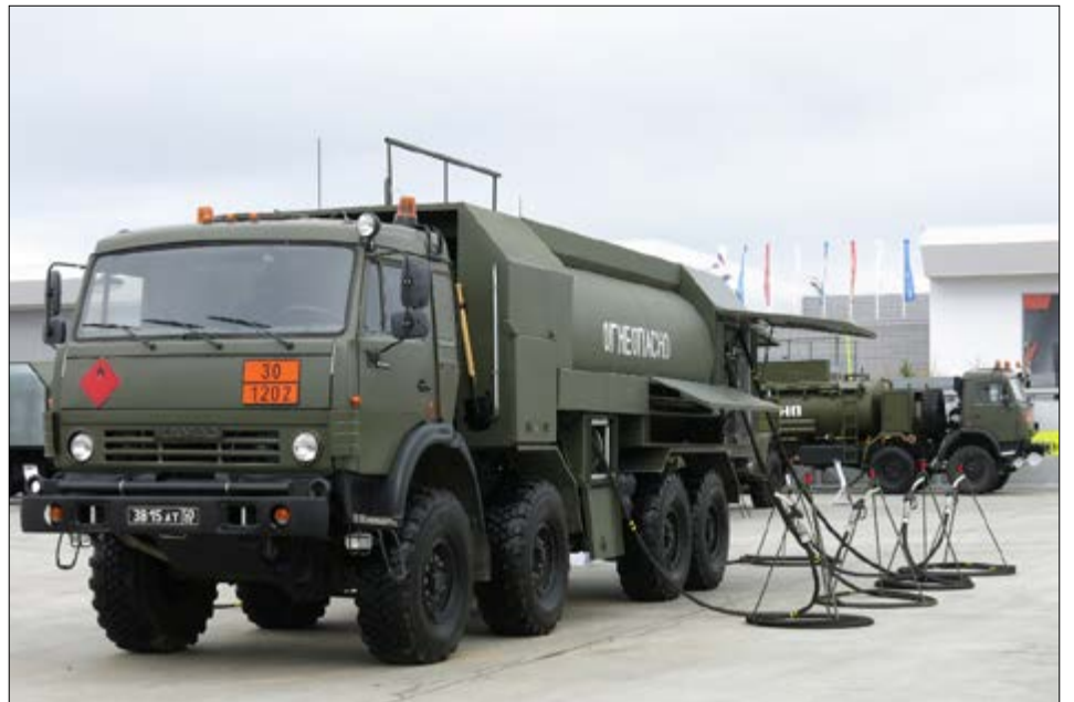
Fuel tanker based on KamAZ-63501 chassis with a capacity of 12000 litres and 10 dispensers. Source: Boevaya mashina via Wikimedia, https://commons.wikimedia.org/wiki/File:ATZ-12-10-63501.jpg , CC BY-SA 4.0
