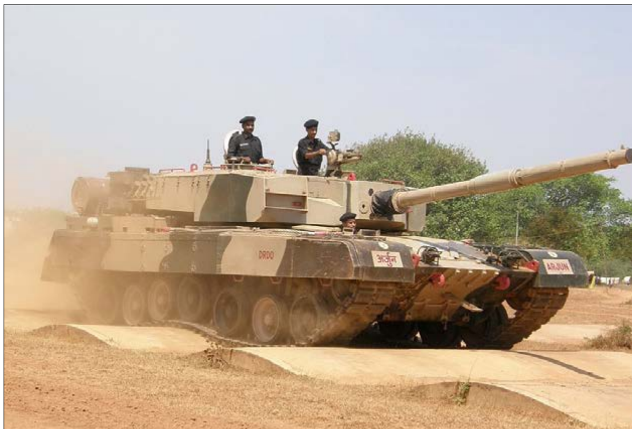
An Arjun MBT being test driven on the bump track at the Central Vehicles Research and Development Establishment (CBRDE) at Avadi, Chennai.
