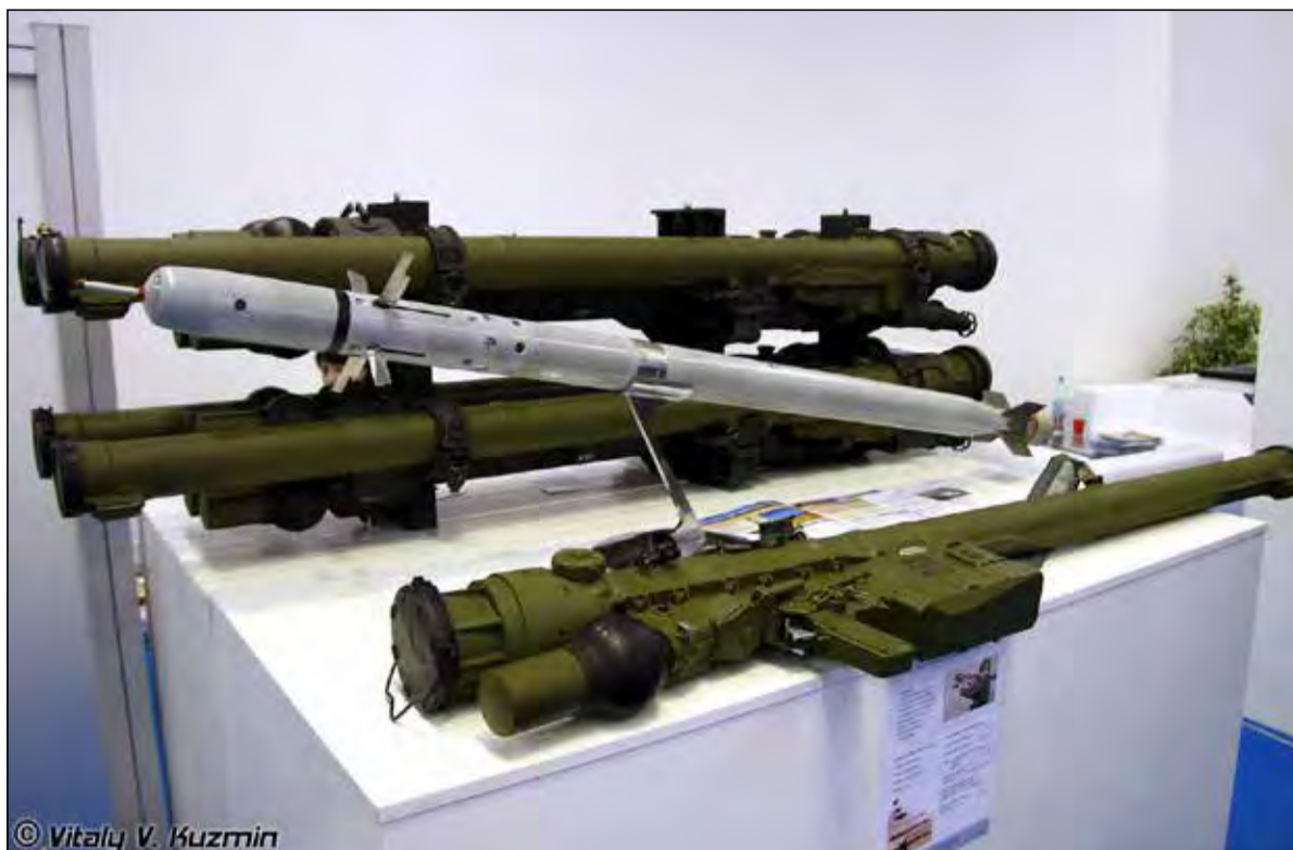
Igla-S MANPADS and Strelets set for firing of missiles of Igla-type MANPADS. Source: Vitaly Kuzmin, https://www.vitalykuzmin.net/Military/Engineering-Technologies-2010/I-BM4LF4Q/A , CC BY-NC-ND 4.0
