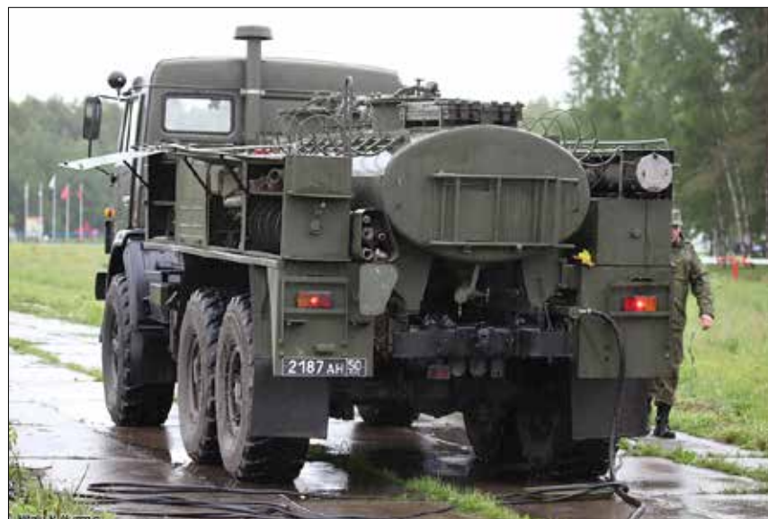
ARS-14KM decontamination and degassing station.
