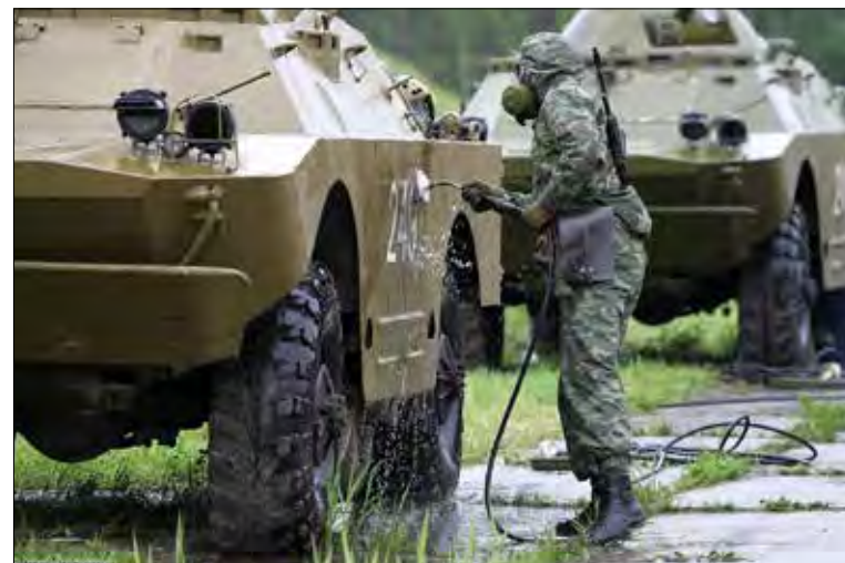
Decontamination of armored vehicles with ARS-14KM decontamination and degassing station.
