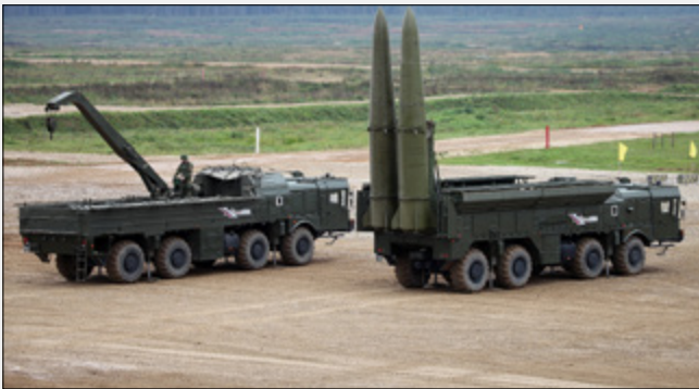
Transporter Erector Launcher (TEL) with 9M723K5 Short Range Ballistic Missiles and Transloader of the Iskander-Mt
