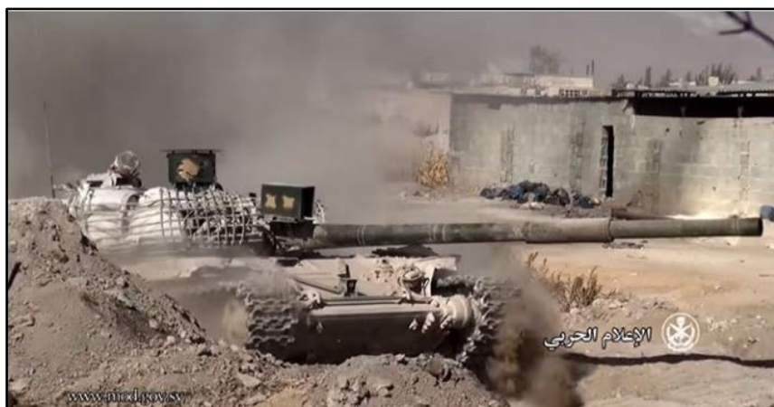
Figure 2. Sarab-2 mounted on a Syrian T-72 toward the end of 2016
