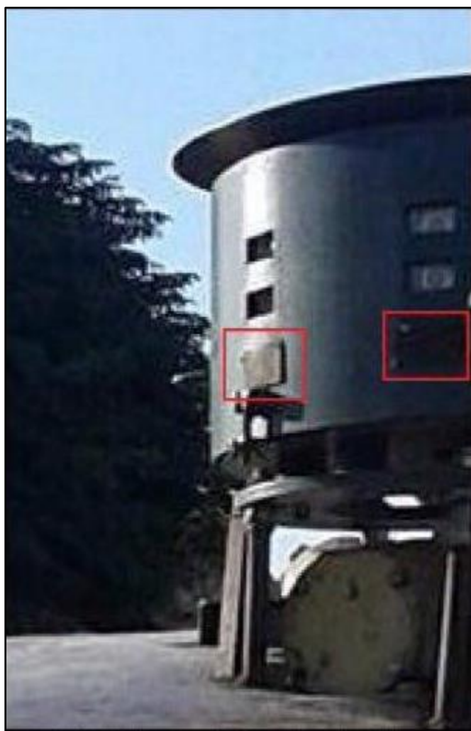
Figure 5. Sarab-3 system with 360 degree slew capability, stacked IR light sources, and possibly laser diodes
