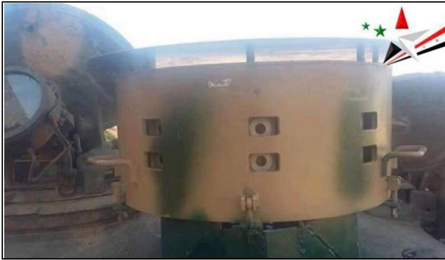
Figure 3. A close-up view of the Sarab-2 system , featuring stacked IR diodes and protective shield
