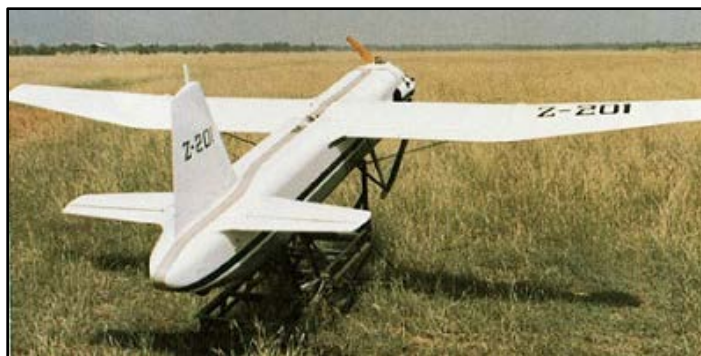
Figure 3. Chinese ASN-104 UAV; the wing and vertical stabilizer have 201 markings, but aircraft characteristics cross-referenced with open-source databases confirm this is an ASN-104
