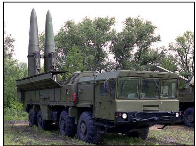
Figure 4. The SS-26 is a short-/medium-range ballistic and cruise missile system; the ballistic missile can perform dramatic terminal phase maneuvers, intended to defeat anti-ballistic missile interceptors
