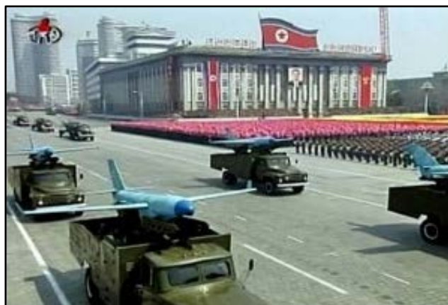
Figure 1. Soviet/Russian Zil-130 truck with UAV launch capability (left) and assessed North Korean one-way strike UAVs, similar to an MQM-107D, on Zil-130 truck chassis (right)
