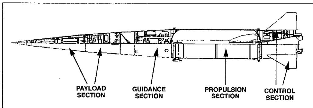
**Mobility.** These missiles employ a high-atmospheric or exo-atmospheric ballistic trajectory to reach the target. Most TBMs follow a set course that cannot be altered after the missile has burned its fuel. However some have the capability for non-ballistic trajectories and precision maneuver. Ballistic missiles have three categories of propellant for engines, which are liquid, hybrid, or solid, effect the distance a missile can travel and the CEP, or accuracy.
