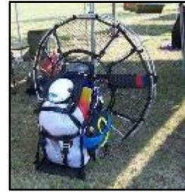
When linked with paragliders, paramotors transform them into **powered paragliders (PG)** to fly 100 kilometers on a tank of gas. Paramotors for paragliders need a power range of only 15 to 30 hp. The equipment can be set up in 15 minutes. Disassembly into 3-4 parts takes about 3 minutes. Flight speed is 32-40 km at 150-5,500 meters altitude. They generally cannot launch from standstill.
