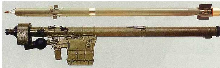
SA-16 MISSILE, AND LAUNCHER WITH PROTECTIVE PAD AND MISSILE CAP FOR TRANSPORT
