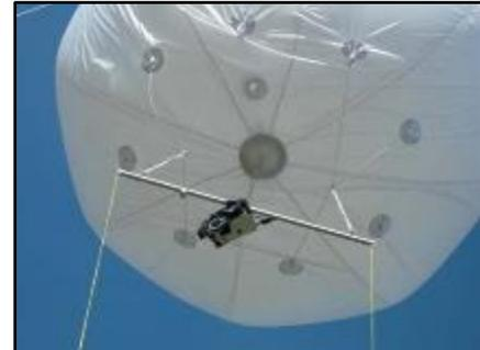
As airships become better-controlled and more stable, other sensors can be added to the payload. An airship could be used in tactical reconnaissance units to mount a small light-weight radar antenna, such as on the FARA-1E (Vol 1, pg 4-29). The Israeli Speed-A stabilized payload system with automated EO/thermal imager and laser rangefinder fits on lightweight airships.
