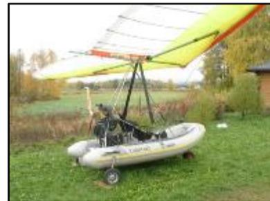
throughout Asia, Europe, and in the U.S. The FIB 2001 Flying Inflatable Boat is an upgraded design using a Lomac RIB hull and weighting 58 kg. It is fitted with a 48-hp Rotax 503 twin-cylinder 2-stroke engine selected for noise suppression. Other FIBs include the 503 (right), with a tandem overhead wing.
