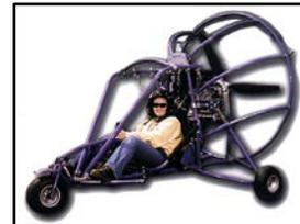
lower stall speeds, and can use unpaved areas as well. One example of a commercial trike is the Powrachute Sky Rascal. The one-seat craft weighs 105/117 kgs, with 40 or 52-hp engine, max payload of 136/159 kgs, and air speed of 67-90 km/hr. Typical trike specifications are as follows:
