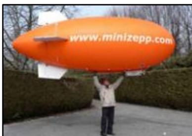
Mini-zepp blimps come in sizes 6-13 m, for use as aerostats or as dirigibles. The dirigibles include 2 electric motors and a gas-powered motor. Options include a video head and HF transmission system. In event of a power failure, a cable drops to the ground for recovery.
