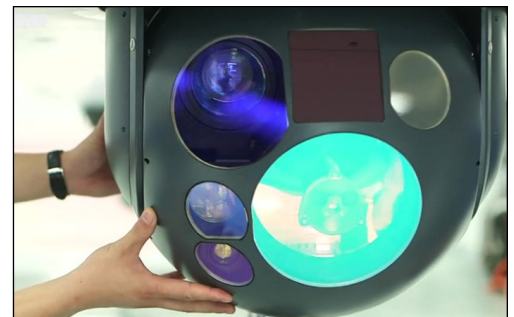
Figure 4. BZK-005/Variant Gimbal with Seven Different Sensors
