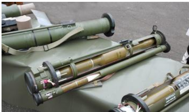
Figure 2. Cutaway of 105-mm and Decoy RPGs
