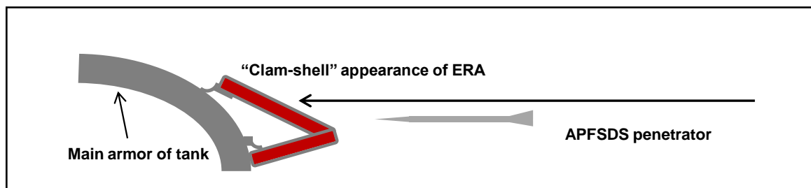
Simplified image of Kontakt-5 explosive reactive armor
