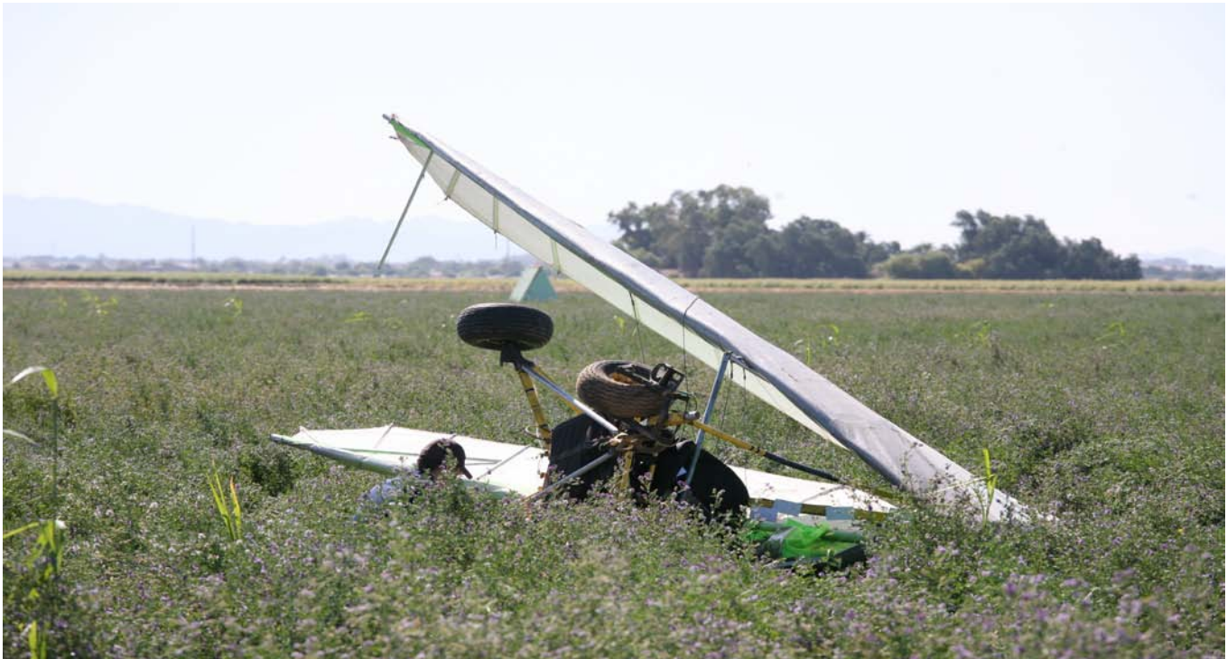
Ultralight crashes like this one are common as pilots receive minimal training, fly into wires and power lines, or simply land too hard (Photo courtesy of U.S. Customs and Border Protection).
