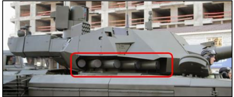
Figure 5. Afghanit APS launchers (outline) turret right-side
