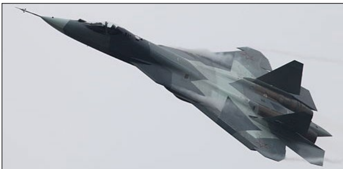
The first PAK FA prototype conducts a test flight. Early prototypes had minimal onboard systems and engines taken from the Su-27 family of aircraft.
