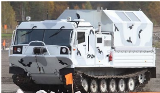
TM-140A amphibious, all-terrain, tracked, Arctic cargo/personnel carrier
